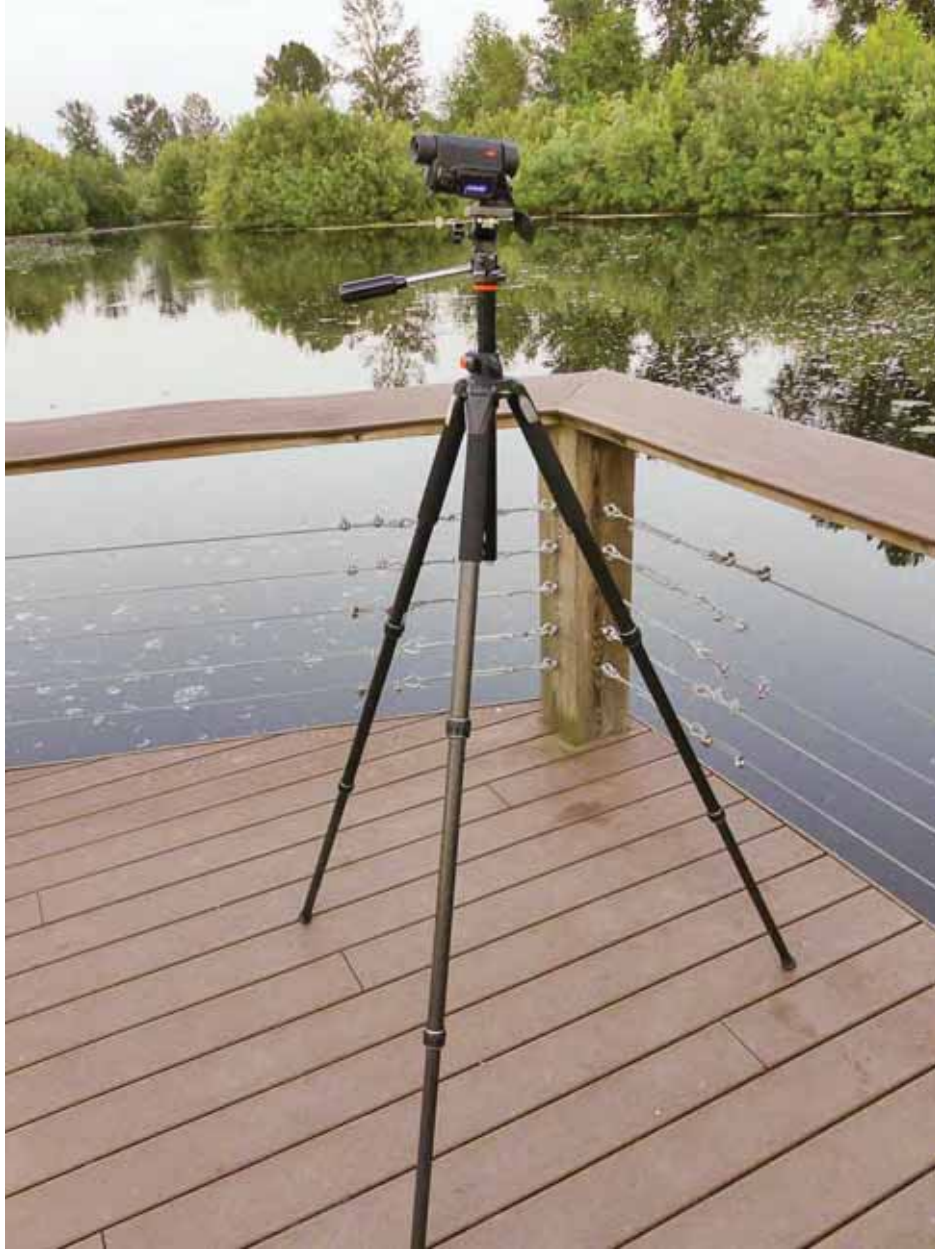
26 - Thermal monocular set up on a tripod to view and record bat foraging in and around a lagoon.
