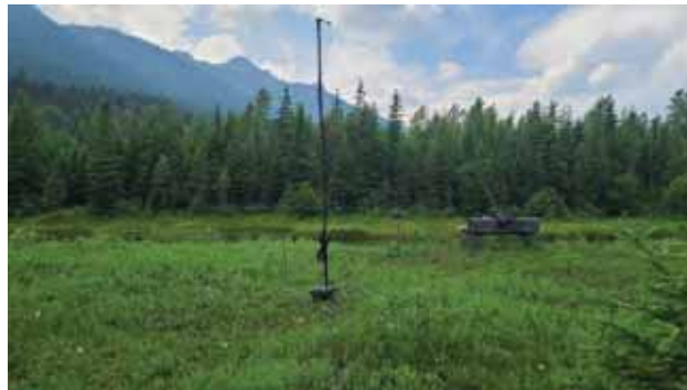
14 - Stationary acoustic detector setup for NABat monitoring. Photo: E. Low.
