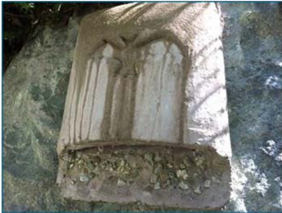
29 - ARR made of concrete fibre and rock crush
