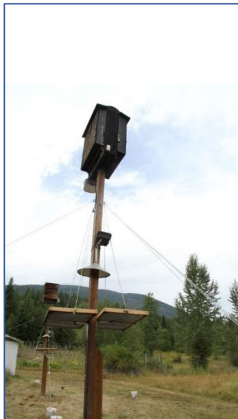
Figure 12. Above Left: Bat boxes with guano traps, roost Loggers, occupancy monitor and HOBO logger. Credit: S. Dulc; Above Right: Photo of tractor harp trap. Credit: L. Mills
